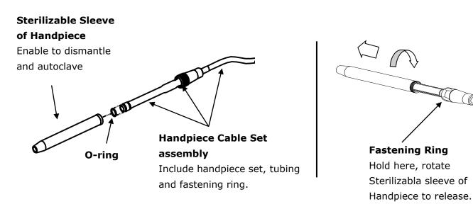
To take off the Sterilizable sleeve of handpiece, please hold the fastening ring, and rotate the sleeve counterclockwise from handpiece cable set assembly. **Note: Avoid rotate or twist the handpiece Cable .**
