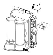
Turn the pump set moderately in the direction of counterclockwise at about 30 degree. Then pull out the complete used pump set with tubing.
