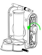
3. Reverse the procedure above, replace with a new tubing pump set.
