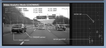
LEADAI fusion technology uses video analytics technology to identify the vehicles and detect lanes based on the given ROI.
